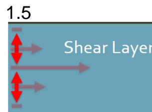
This gradient creates a shear environment where the DRA structure could deform or even break.
