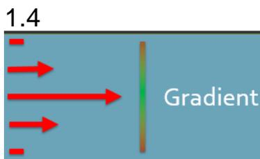
This creates a gradient – the fluid in the middle is moving fast and the fluid at the walls is not moving at all.
